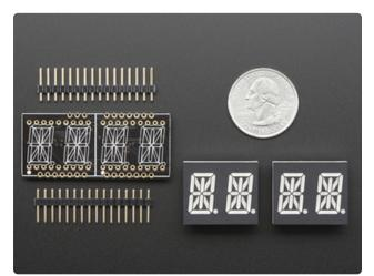
When you buy a pack from Adafruit, it comes with the fully tested and assembled backpack as well as a two 14-segment dualdisplays in one of the colors we provide (say, red, yellow, blue or green). You'll need to solder the matrix onto the backpack but it's an easy task.
