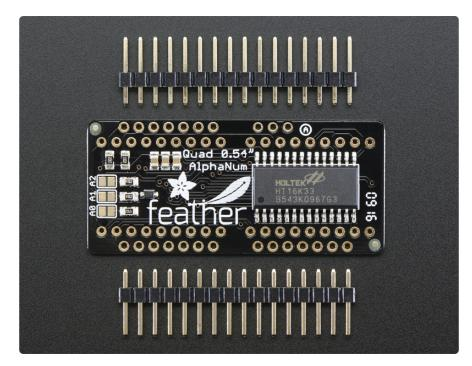
The LEDs themselves do not connect to the Feather. Instead, a matrix driver chip (HT16K33) does the multiplexing for you. The Feather simply sends i2c commands to the chip to tell it what LEDs to light up and it is handled for you. This takes a lot of the
