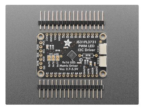
To get you going fast, we spun up a custom-made PCB in the **STEMMA QT** form factor (https://adafru.it/LBQ), making it easy to interface with. The STEMMA QT connectors (https://adafru.it/JqB) are compatible with the SparkFun Qwiic (https://
