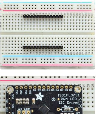
Prepare the header strip: Cut the strip to length if necessary. It will be easier to solder if you insert it into a breadboard - long pins down
