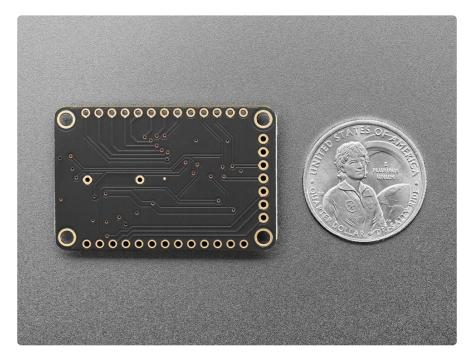
The IS31FL3731 is a nice little chip - it can use 2.7-5.5V power and logic so it's flexible for use with any microcontroller. You can set the address so up to 4 matrices can share an I2C bus. Inside is enough RAM for 8 separate frames of display memory, so
