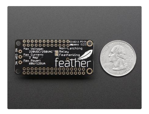
Each FeatherWing comes with a fully assembled and tested PCB, header you can use to attach to your feather. You also get a 3-pin terminal block you can use to wire up whatever you are going to be relay-controlling. Some light soldering is required
