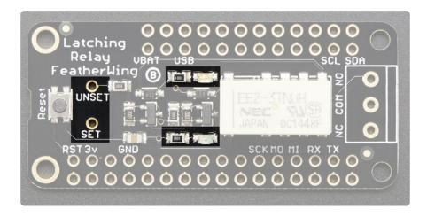
The latching relay uses two pins for control. There is no way to know which 'orientation' the relay is when the Feather turns on, because the relay will latch in the last position it was set to.
